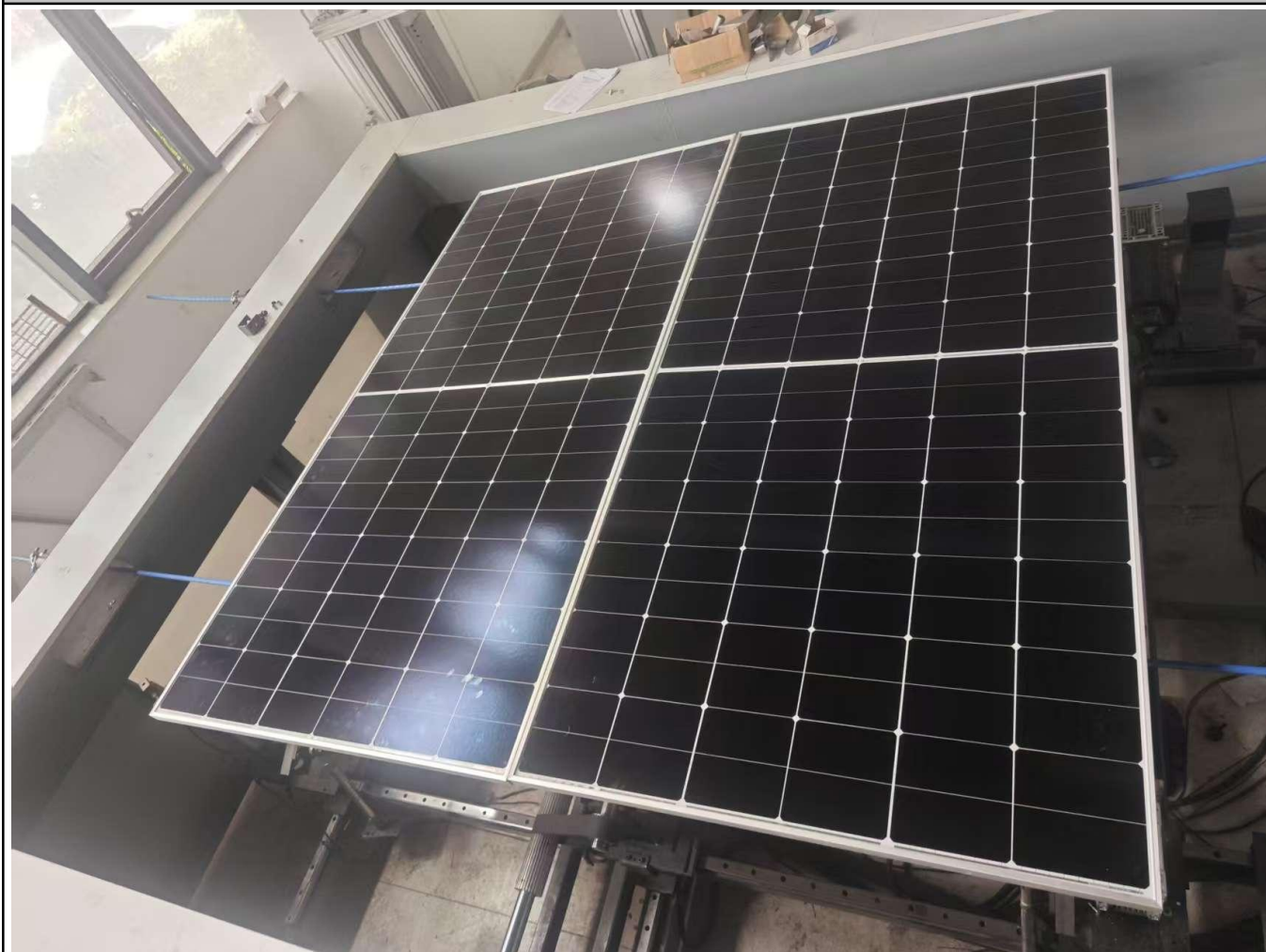
激振疲劳测试安装照
